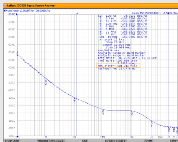
Ultra-Low Phase Noise: 105 fs at 12 kHz to 20 MHz
