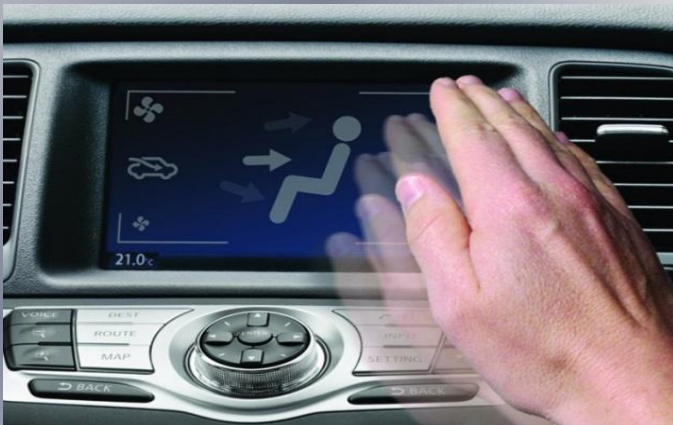
Capacitive Gesture Recognition
