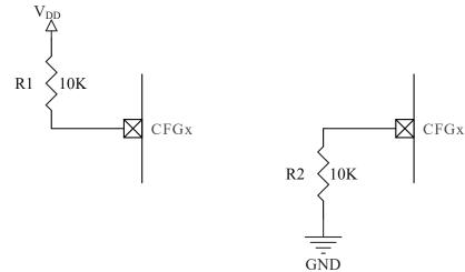
The pull-up/pull-down resistor is a precautionary recommendation, as MTCH1010 will not pull the CFGx neither to the  $V_{DD}$  nor to the GND during the operation.
