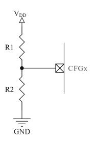
Note: Both R1 and R2 are recommended to be greater than 100K for lower power consumption
