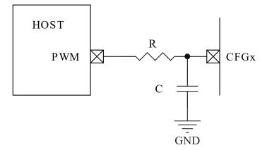
Note: Refer to Application Note 'Using PWM to Generate Analog Outpout (AN538)' for details about how to choose appropriate R and C values
