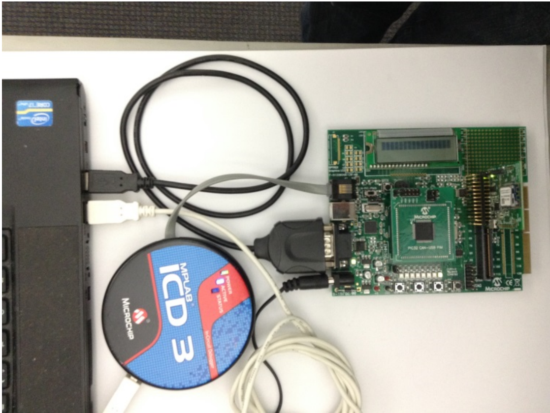
WINC1500 PICtail Module FW Serial Update Using the pic32mz_ef_sk + Starter Kit I/O Expansion Board + pic32mz Starter Kit Adapter Board
