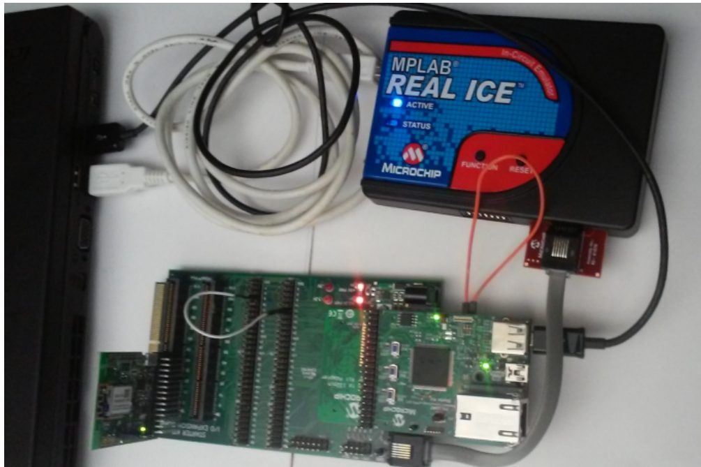
WINC1500 PICtail Module FW Serial Update Using the pic32mz_ef_sk + Starter Kit I/O Expansion Board + pic32mz Starter Kit Adapter Board
