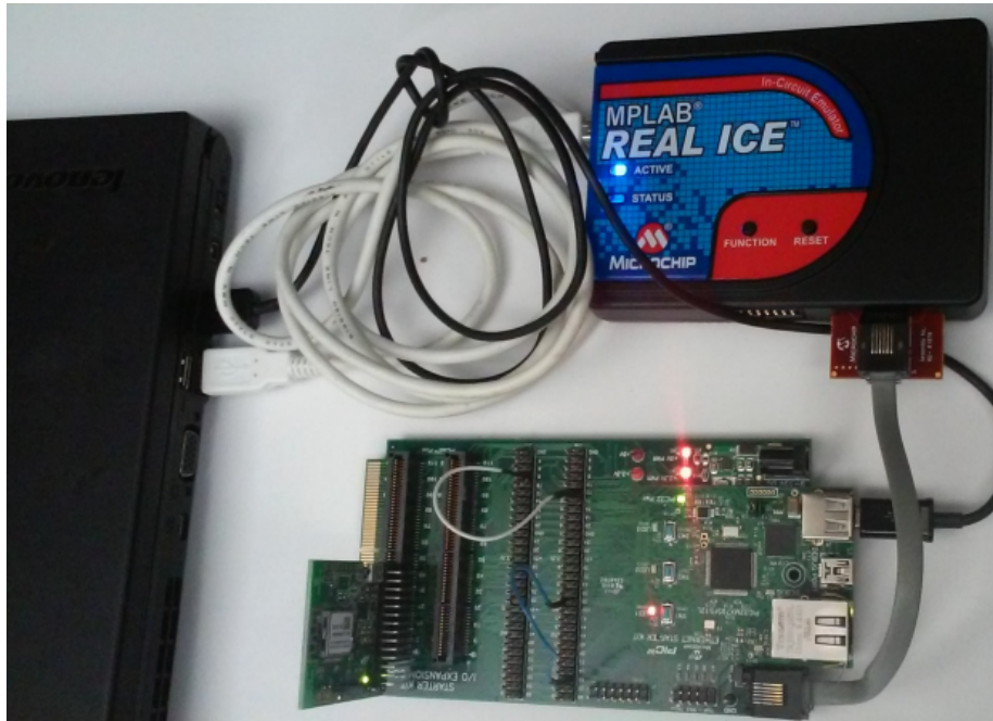
WINC1500 WiFi 7 Click Module FW Serial Update Using the pic32mx795_pim+e16_32
