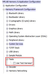
5. Configure the test harness. Refer to the online Help associated with each option for a description of what it means. The test harness directly utilizes a timer (via the Timer PLIB) to provide a timeout capability and OSAL functions, even if no RTOS is selected.
