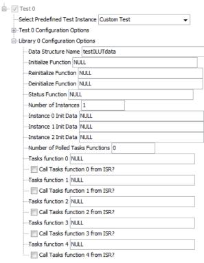
8. Generate the configuration. This will insert the test harness library into your project and generate the necessary test list, initial data structures and other configuration code. You may need to make updates to these later as you develop your tests so that you can easily execute them under control of the test harness.
