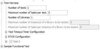
6. Configure each test, entering the names of the test, its required functions and data structure and other information. Note that the MPLAB Harmony installation does provide some predefined tests. These can be selected and used to test supported pre-existing libraries. However, you will normally need to configure a "Custom Test" and fill in all of the required information manually as no predefined test will be provided for a newly created library.
