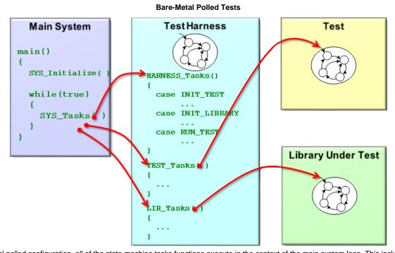
In a bare-metal polled configuration, all of the state machine tasks functions execute in the context of the main system loop. This includes the tasks function for the test harness, the test, and the LUT. However, the test and library tasks are only executed when the test harness state machine permits so that the harness can track and control them.
