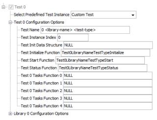
7. Enter the library configuration options for the library under test that is associated with each test. This will include the library's function names and initialization data structure name as well as information on the number of instances, polled and interrupt-driven tasks functions (and associated interrupt details).
