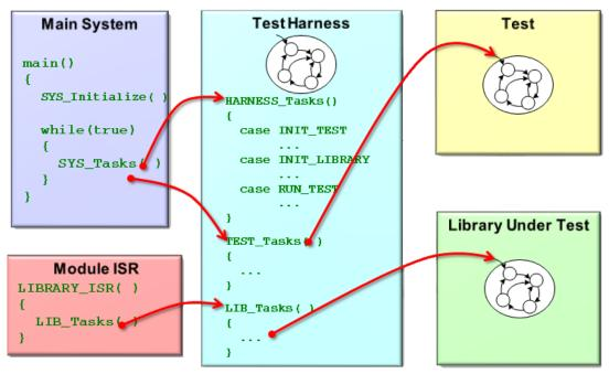
In an interrupt-driven test configuration in a bare-metal environment (with no OS), one or more of the tasks functions for the library under test may run within the context of an Interrupt Service Routine (ISR) that is defined for that peripheral module, depending on what is appropriate for the LUT. These ISR-ready Tasks functions are still called indirectly through the test harness so that it can capture spurious interrupts and manage the execution of the test and LUT.
