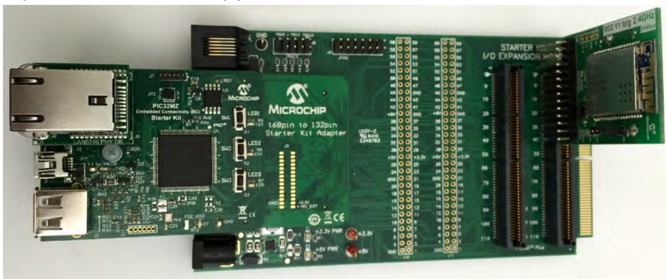
PIC32MZ EC Starter Kit, MRF24WN0MA Wi-Fi PICtail/PICtail Plus Daughter Board, and Starter Kit I/O Expansion Board
