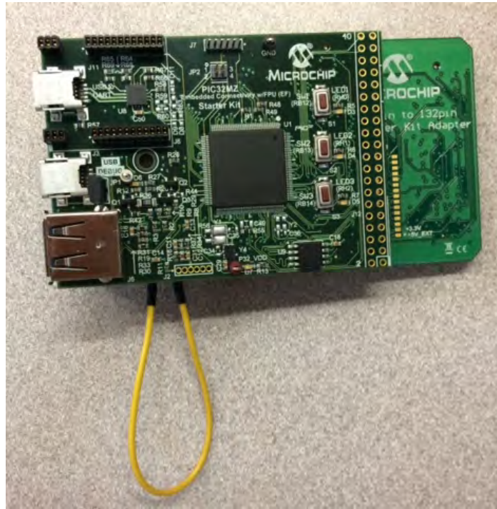
PIC32MZ EF Starter Kit and Adapter Board connected to the Graphics Controller PICtail Plus Epson S1D13517 Daughter Board
