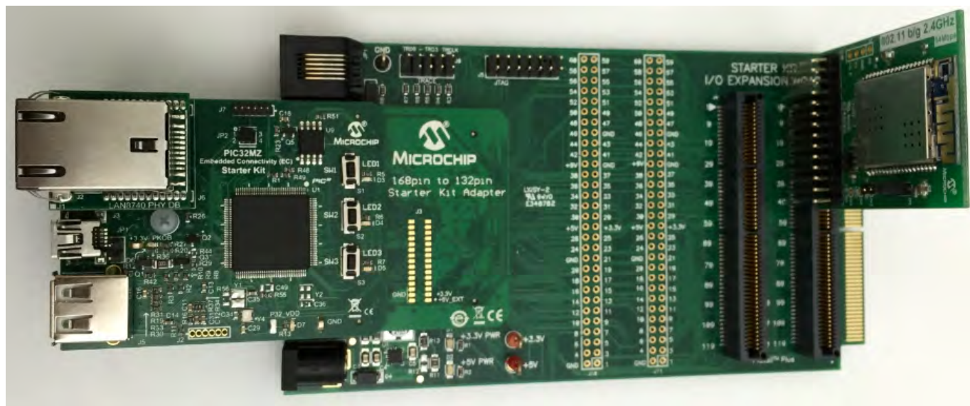
PIC32MZ EC Starter Kit with PIC32MZ2048ECH144, MRF24WN0MA Wi-Fi PICtail/PICtail Plus Daughter Board, and Starter Kit I/O Expansion Board
