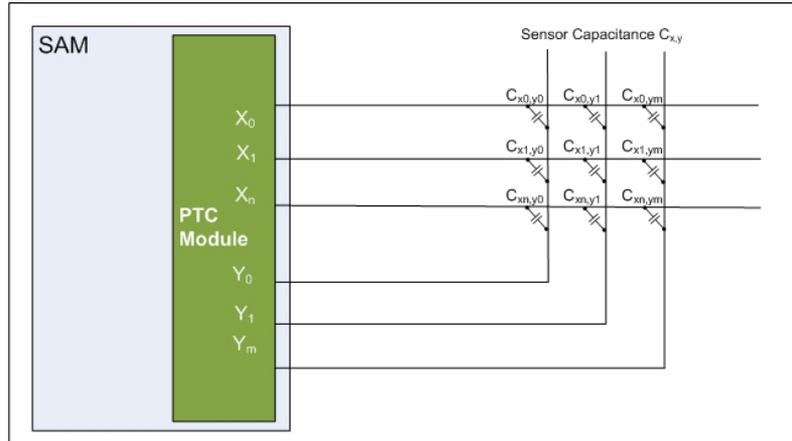
To reduce noise issues due to EMC, use a series resistor with value of 1k $\Omega$  on X and Y lines.
