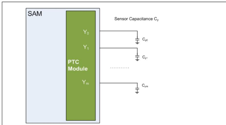
**Figure 2-7. Self Capacitance - Channel to Sensor Mapping**
