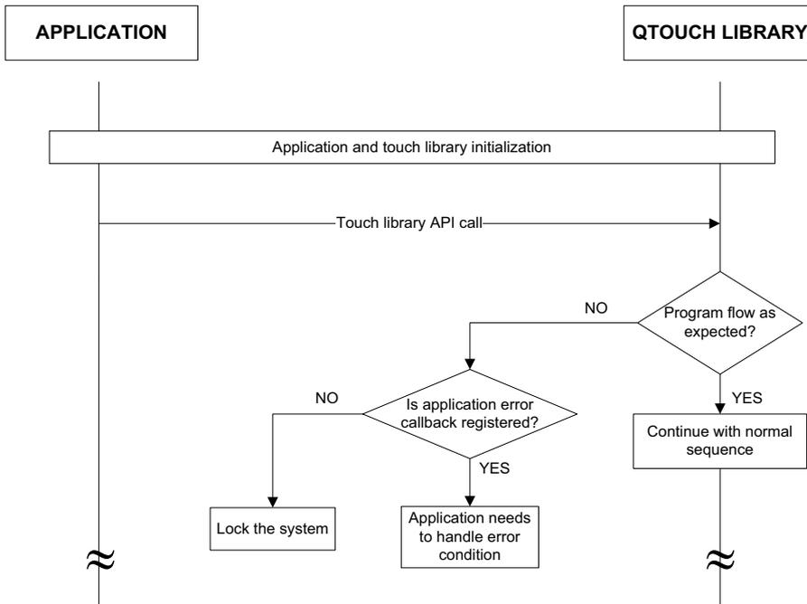
Figure 2-12. Example of a Wrong API Sequence
