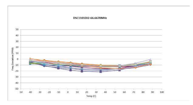
The frequency stability is actually independent of package and output frequency and is fairly constant over the entire temperature range.
