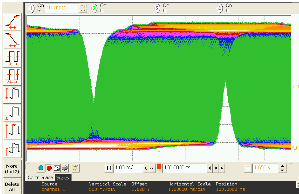
Incoming 100MHz Clock at 10 th Edge After the Trigger
