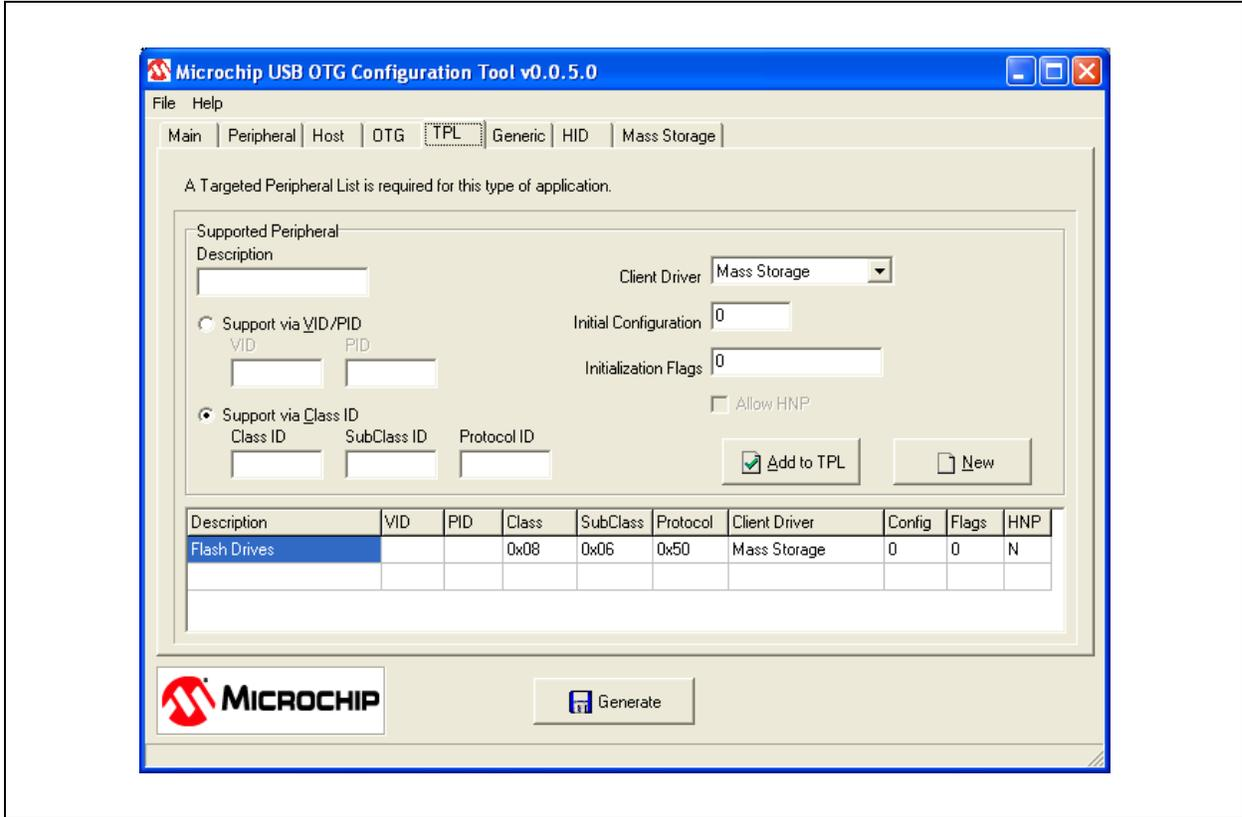
**FIGURE 6: USB CONFIGURATION TOOL, MASS STORAGE TAB**
