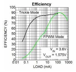
The Figure above shows an efficiency curve. From no load to 100mA, efficiency losses are dominated by quiescent current losses, gate drive and transition losses. By Forcing the MIC2238 into Trickle Mode (/FPWM=High), the buck regulator significantly reduces the required switching current by entering into a PFM (Pulse Frequency Modulation) mode. This significantly increases efficiency at low output currents.
