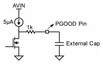
Figure 1. Power Good Circuit
