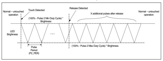
FIGURE 6-4: Pulse 2 Behavior with Inverted Polarity
