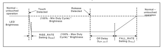
FIGURE 6-8: Direct Behavior for Inverted Polarity
