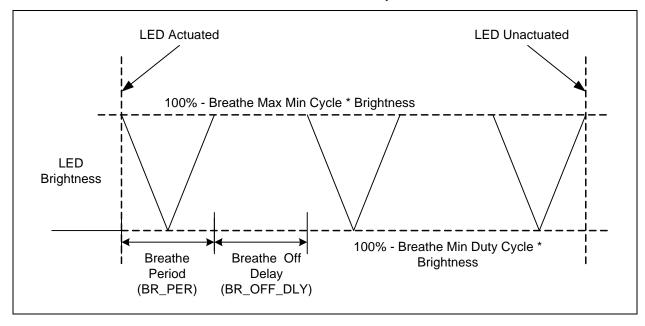
FIGURE 6-6: Breathe Behavior with Inverted Polarity
