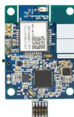
This board driven by SAML21 MCU is packed with sensors and BTLC1000 module on a tiny form factor PCB (40 × 30 mm) to demonstrate the ultra low power capabilities of SAML21 for wearable applications. It runs on coin cell battery and comes with a free android app to provide 3D plot, step count, motion and environment sensing information.
