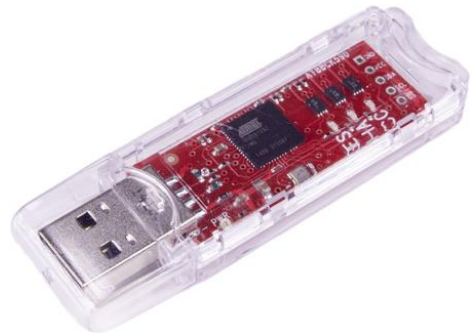
Figure 2-2. AT88CK590 Demo-evaluation Kit
