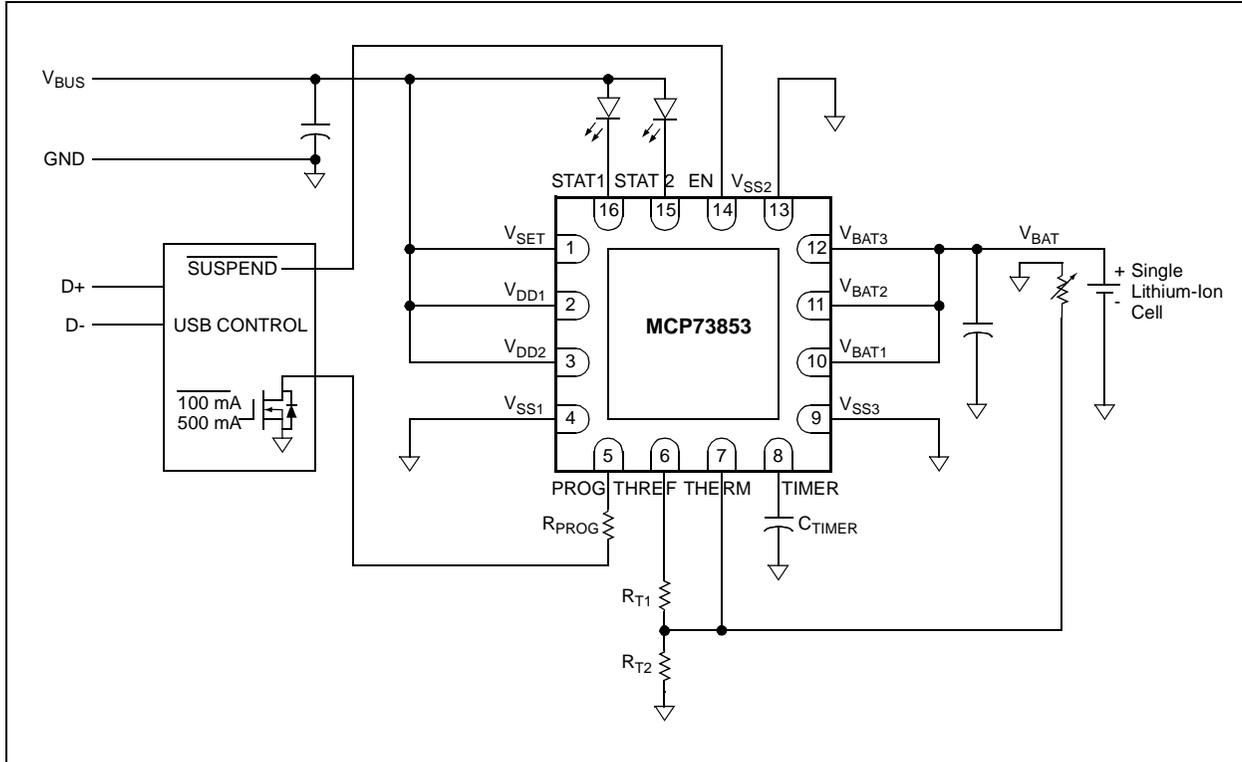
**FIGURE 2:** USB-powered, Single-cell, Li-Ion/Li-Polymer Battery Charger with Cell Temperature Monitoring.
