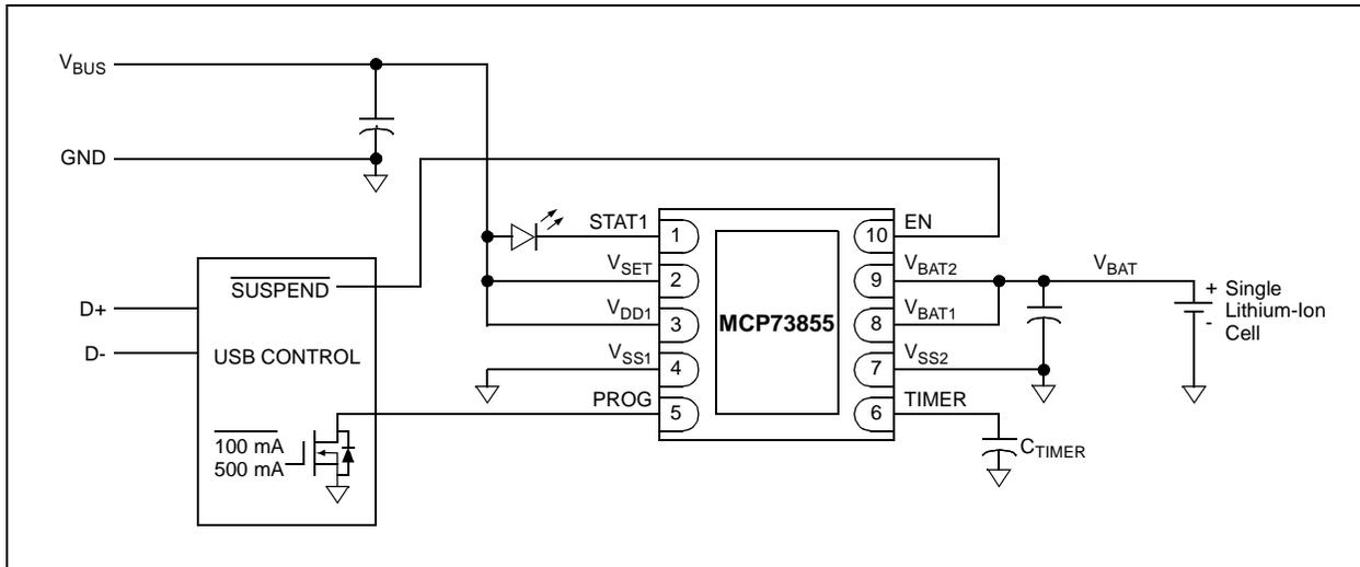
**FIGURE 3:** Small PCB Area USB-powered, Single-cell, Li-Ion/Li-Polymer Battery Charger
