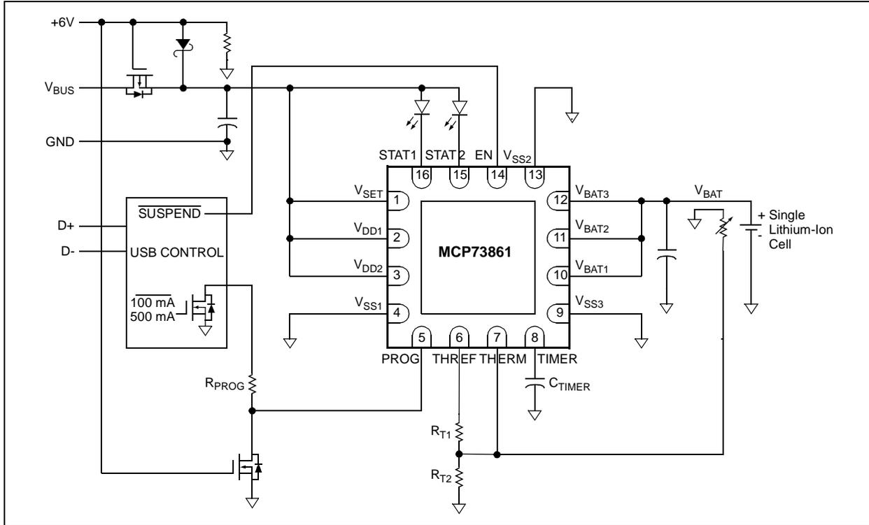
**FIGURE 4:** USB-powered or Externally-powered, Single-Cell, Li-Ion/Li-Polymer Battery Charger with Cell Temperature Monitoring.
