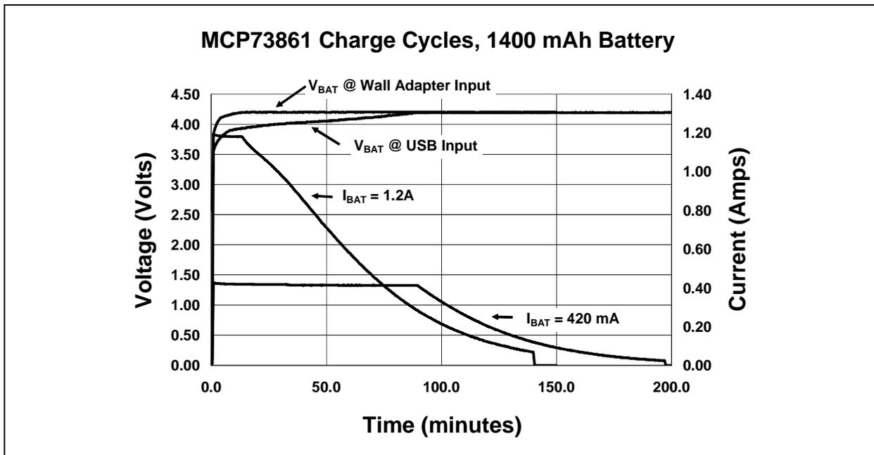
**FIGURE 5:** MCP73861 Charge Cycle Waveforms.
