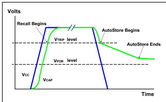
When power is removed and  $V_{CC}$  falls,  $V_{CAP}$  voltage will fall as well, but when the internal power rail falls below  $V_{TRIP}$ , the device automatically disconnects the switch between  $V_{CAP}$  and  $V_{CC}$ , and this allows the capacitor to provide the power, independent of  $V_{CC}$ , for the duration of the AutoStore.
