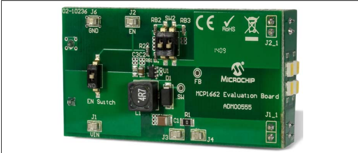
FIGURE 17: MCP1662 Evaluation Board – Flashlight with four LEDs driven by switch to three current levels (30 mA, 60 mA, 90 mA).
