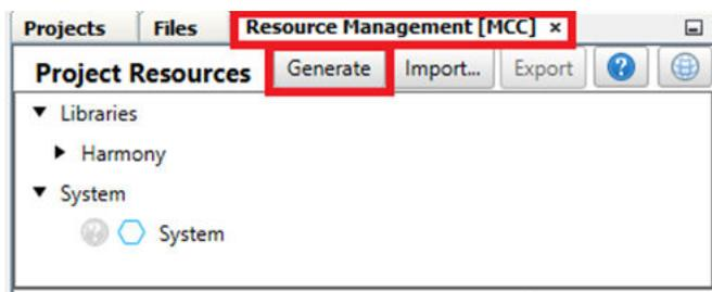
**Note:** The generated code will add files and folders to the 32-bit MCC Harmony project. In the generated code, notice the Peripheral Library files that are generated for the Real-Time Clock (RTC), External Interrupt Controller (EIC), PORT, SERCOM1 (as USART), and DMA peripherals are added in the project. The MCC also generates the `main.c` files in the project.
