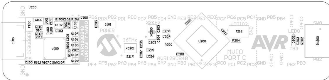
Figure 8-3. AVR128DB48 Curiosity Nano Assembly Drawing Bottom
