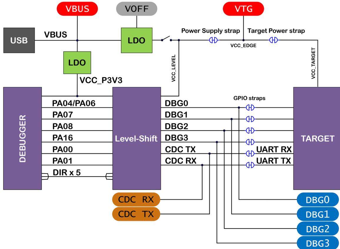
Figure 8-6. On-Board Debugger Connection Cut Straps
