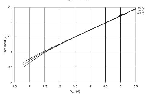
Figure 19-47.  $V_{IH}$ - $V_{IL}$ : Input Hysteresis vs.  $V_{CC}$  (I/O Pin)
