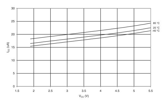
Figure 19-18. ADC Current vs. V<sub>CC</sub>
