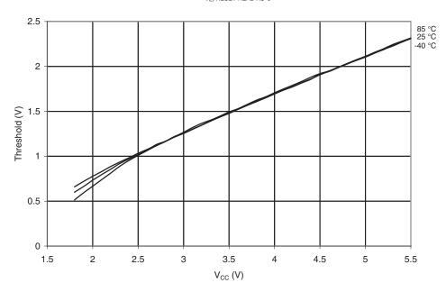
**Figure 19-50.**  $V_{IH}$ - $V_{IL}$ : Input Hysteresis vs.  $V_{CC}$  (Reset Pin as I/O)
