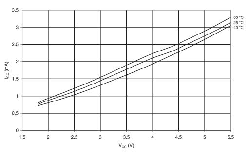
$\textbf{Figure 19-5.} \quad \text{Active Supply Current vs. } V_{\text{CC}} \text{ (Internal WDT Oscillator, 128 kHz)}$
