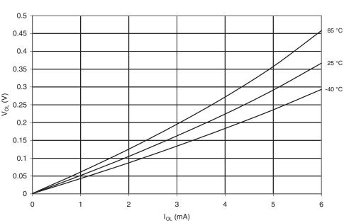
I/O PIN OUTPUT VOLTAGE vs. SINK CURRENT  $V_{CC} = 1.8V$
