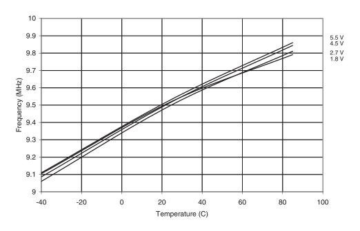
Figure 19-60. Calibrated 9.6 MHz RC Oscillator Frequency vs. V<sub>CC</sub>
