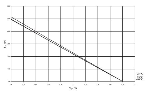
Figure 19-22. Pull-up Resistor Current vs. Input Voltage (I/O Pin, V<sub>CC</sub> = 3V)
