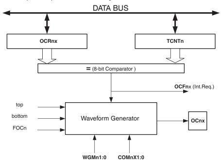
Figure 11-3. Output Compare Unit, Block Diagram
