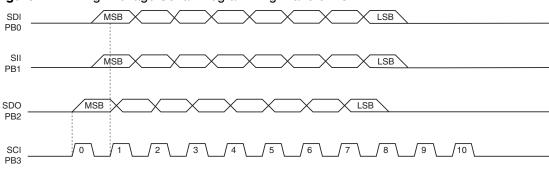
Figure 17-4. High-voltage Serial Programming Waveforms
