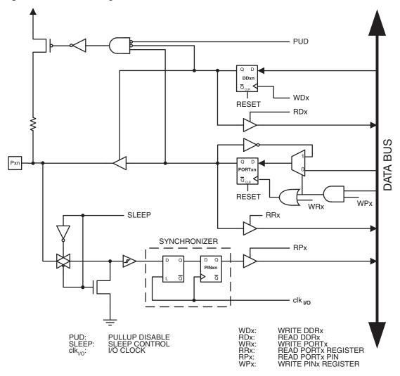
Note: 1. WRx, WPx, WDx, RRx, RPx, and RDx are common to all pins within the same port.  $clk_{I/O}$ , SLEEP, and PUD are common to all ports.
