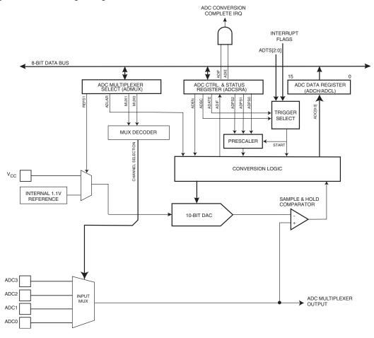
The ADC is connected to a 4-channel Analog Multiplexer which allows four single-ended voltage inputs constructed from the pins of Port B. The single-ended voltage inputs refer to 0V (GND).
