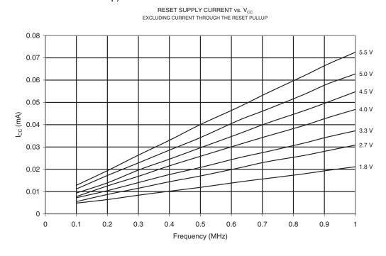
**Figure 19-16.** Reset Supply Current vs. V<sub>CC</sub> (1 - 20 MHz, Excluding Current through the Reset Pull-up)
