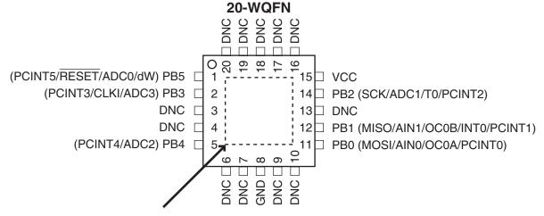
NOTE: Bottom pad should be soldered to ground.
