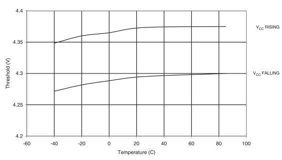
Figure 19-52. BOD Thresholds vs. Temperature (BODLEVEL is 2.7V)
