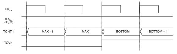
Figure 11-9 shows the same timing data, but with the prescaler enabled.
