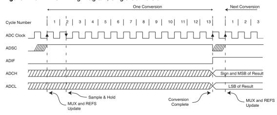
Figure 14-5. ADC Timing Diagram, Single Conversion
