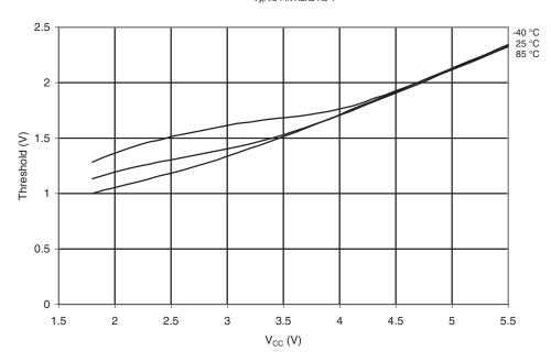
Figure 19-56.  $V_{IL}$ : Reset Input Threshold Voltage vs.  $V_{CC}$  (Reset Pin Read as '0')
