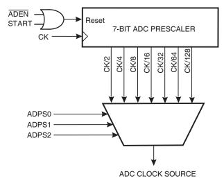
The ADC module contains a prescaler, which generates an acceptable ADC clock frequency from any CPU frequency above 100 kHz. The prescaling is set by the ADPS bits in ADCSRA.
