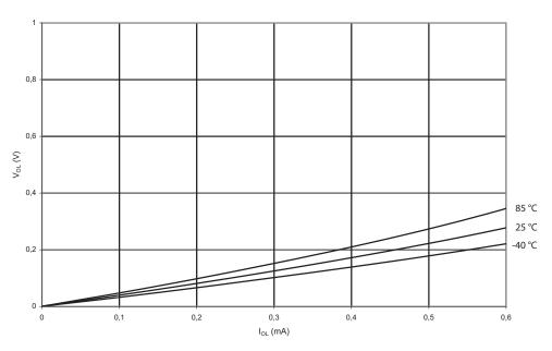
Figure 19-43.  $V_{OL}$ : Reset Pin as I/O, Output Voltage vs. Sink Current ( $V_{CC} = 3V$ )
