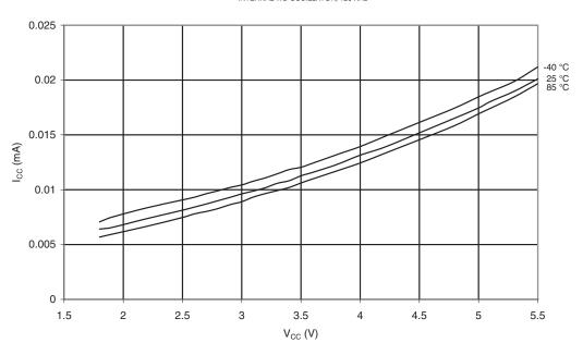
Figure 19-12. Idle Supply Current vs. V<sub>CC</sub> (32 kHz External Clock)
