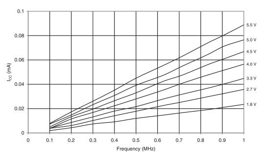
Figure 19-8. Idle Supply Current vs. Frequency (1 - 20 MHz)
