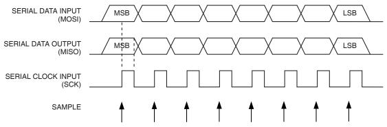
**Table 18-9.** Serial Programming Characteristics,  $T_A = -40$ °C to +85°C
