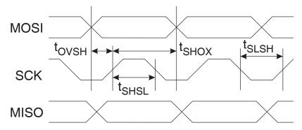
Figure 18-4. Serial Programming Waveform
