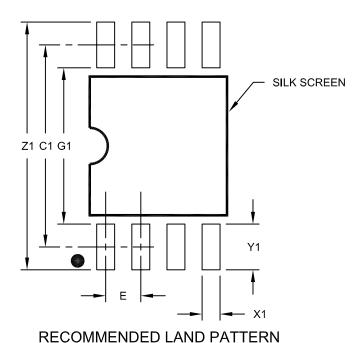
**MILLIMETERS** Units **Dimension Limits** MIN MOM MAX 1.27 BSC Contact Pitch Ε 9.00 Overall Width Z1 Contact Pad Spacing 7.30 C1 Contact Pad Width (X8) 0.65 Χ1 Contact Pad Length (X8) 1.70 Υ1 Distance Between Pads G1 5.60 Distance Between Pads G 0.62
