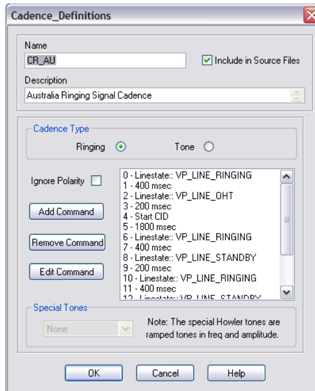
Figure 10-7. Profile Wizard – Ringing Cadence Profile Example
