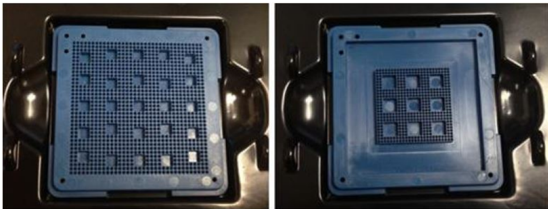
Figure 3-3. CG624 in Its Carrier (Left) and CG1152 in Blue Carrier with 1.0 mm Column Pitch (Right)
