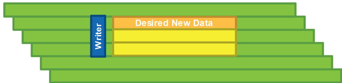
Figure 3 • Overwriting Existing Data on an SMR Drive
