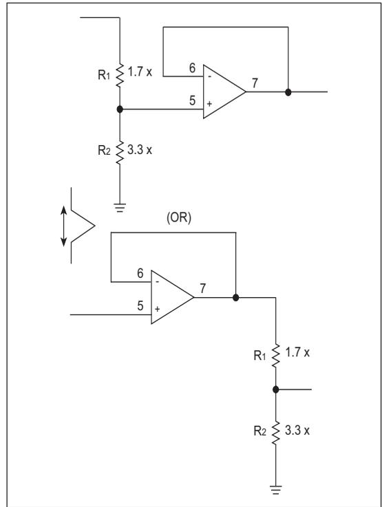
If the resistor divider is before the unity gain follower, then the lowest possible impedance is provided for the 3.3V circuits. Also, the op amp can be powered from 3.3V, saving some power. If the X is made very large, then power consumed by the 5V side can be minimized.
