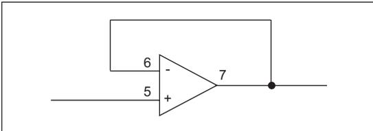
This circuit will output the same voltage that is applied to the input.
