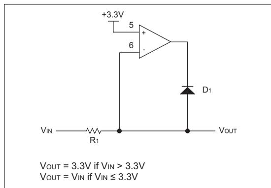
Because the clamping is performed by the op amp, there is no affect on the power supply. The impedance presented to the low voltage circuit is not improved by the op amp, it remains  $R_1$  in addition to the source circuit impedance.
