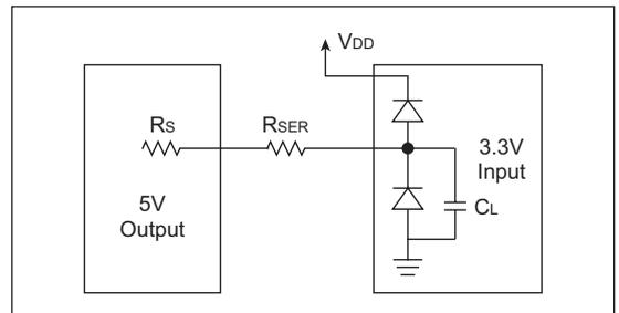
If the clamping diodes are not present, a single external diode can be added to the circuit as shown in Figure 10-2.
