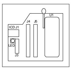
The UPM does not have a separate power source. Power is supplied to the UPM by the development tool in use. MPLAB ICD 2 uses a 9V DC power supply (AC162039). The MPLAB PM3 uses a 3V/5V DC power supply (ACICE0401).
