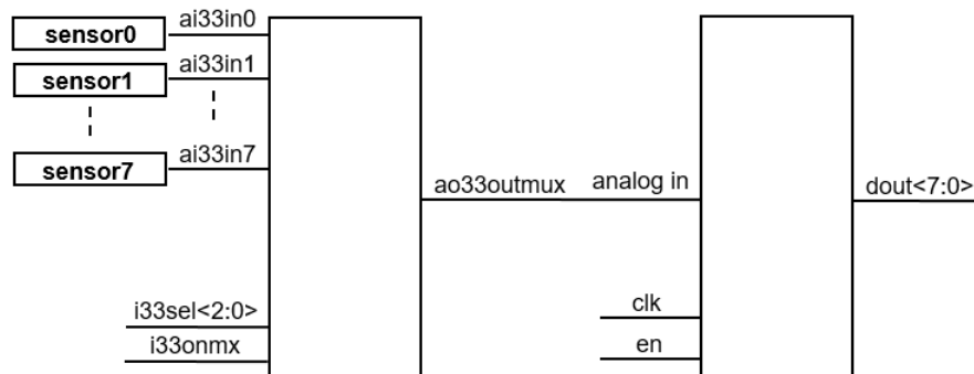
Figure 5-1. Multiplexing Analog Inputs to an ADC
